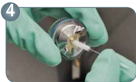
When cleaning the nozzle components, please make sure that metal parts of brushes do not damage the nozzle set.
